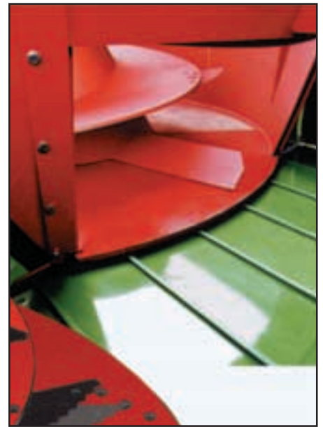
An additional clearing device at the lower part of the mixing auger guarantees a fast and constant discharge of the fodder mixture
