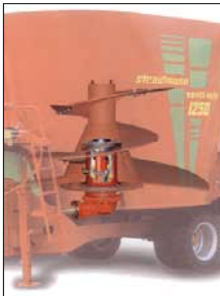
The auger is driven by an extremely robust planetary reduction gearbox set at 26 RPM standard speed on the 1050. An optional secondary gearbox provides a 30% lower start-up speed - intended for lower powered tractors.
