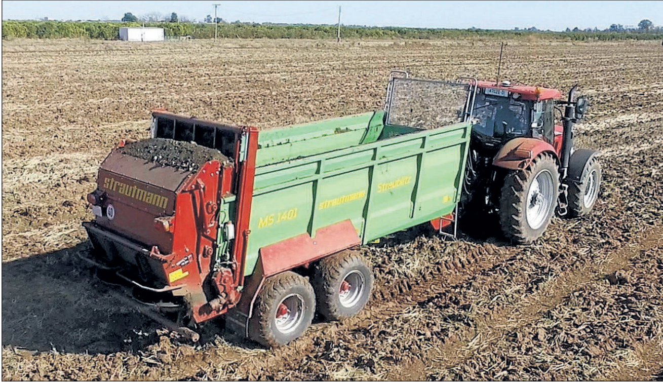
The Strautmann MS 1401 Universal Spreader can spread a wide range of organic and mineral material from fine compost or crumbly lime to heavy manure.
